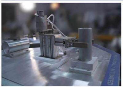
This table is equipped with pneumatically actuated pick and place unit which picks up first pipe and places it inside the second pipe. Pick and place arrangement is controlled through PLC. Robot then carries out 3 dimensional circular welding of two hollow pipes.
