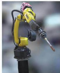
Industrial Welding Robocell from Hytech Didactic consists of 3 individual experiment tables and an industrial welding robot with minimum reach of 1000mm. Central Control Unit equipped with PLC, HMI and IIOT is integrated with Welding Robot. Robot can be programmed from a teach pendant or from an offline programming software which can also act as a digital dynamic twin.
