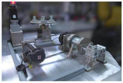
This table is provided with two separate automated welding arrangements. Setup I consists of an indexing table equipped with AC Servo Motor. User can program Servo Motor from PLC and integrate the automation process with Welding Robot to carry out automated welding of jobs. Robot can weld one job on the indexing table and wait for the servo motor to be indexed from PLC and then carry out the welding of next job at the same location.
