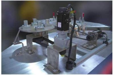
This table is provided with two separate automated welding arrangements. Setup 1 consists of an indexing table equipped with AC Servo Motor. User can program Servo Motor from PLC and integrate the automation process with Welding Robot to carry out automated welding of jobs. Robot can weld one job on the indexing table and wait for the servo motor to be indexed from PLC and then carry out the welding of next job at the same location.
