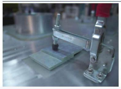
This table is provided with mechanical clamping arrangements. Various types of joints can be welded on this table.
