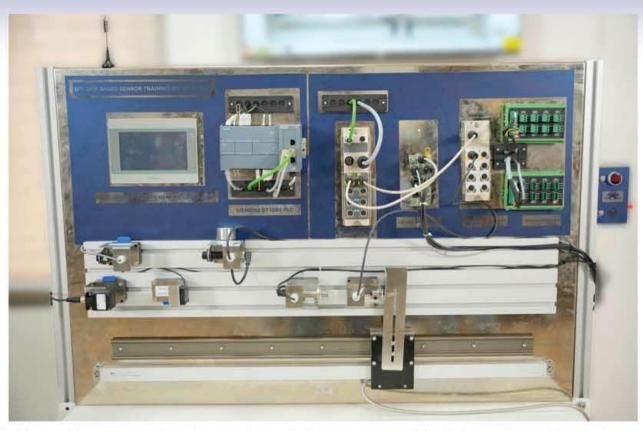
This kit enables user to interface various digital, analog and io link sensors with relative ease. Architecture of Sensor and IIOT training kit is arranged in such a way that any and every sensor such as vision sensor, LiDar sensor or any other advanced sensor can be integrated with this training kit.
