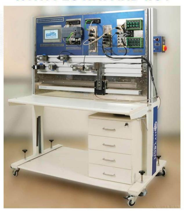
Sensor Training kit from Hytech Didactic is designed to provide users with hands on experience on latest sensor technologies which can be easily upgraded in future. This kit is equipped with various sensors based on io link technology which are integrated with PLC and HMI.
