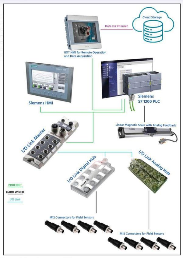
No. of Sensors that can be connected: 64
