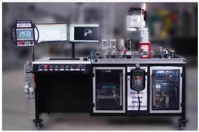
SCARA Cell integrated with PLC and IIOT HMI provides hands on experience on industrial SCARA applications. Color sensor with IO link connectivity and Load cell with amplifier are provided for sorting and palletizing application in integration with SCARA – PLC and IIOT HMI.
