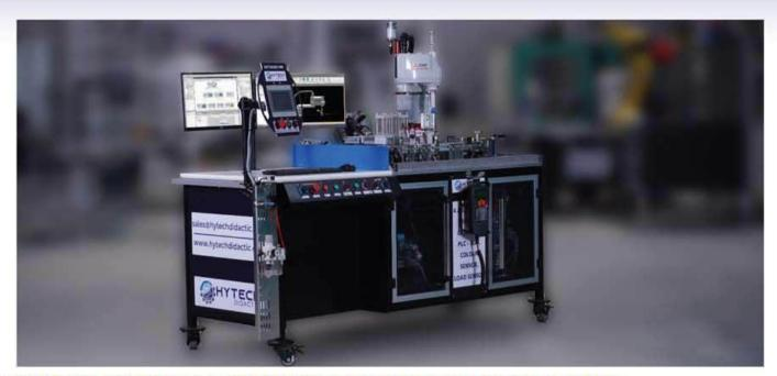
PROCESS 1: WEIGHT BASED SORTING WITH SCARA (PLC AND HMI INTEGRATION)
