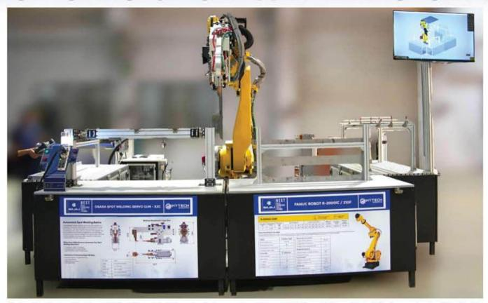
Hytech Didactic Spot Welding Cell is a training cell with a SPOT welding Robot integrated with PLC – HMI and IIOT. Participants can carry out automated welding in integration with Servo Motor as well. Three experiment tables provide hands on experience on horizontal as well as vertical spot welding. Separate Central Control Unit with workstation and dual monitors provides easy access for the robotic as well as PLC programming.
