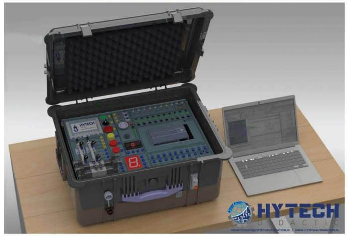
Hytech Didactics' Briefcase PLC and HMI Training Kit is equipped with state-of-the-art products from Siemens S7 1200-1215 PLC and KTP 400 HMI.
