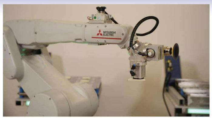
The industrial Robotic process includes pick up of the job from storage by a robot and detecting its shape through vision inspection. Depending on the input received from vision system, first robot carries out the deburring application and second robot can carry out the polishing application. Depending on user requirement, second robot can carry out engraving application. Both robots can work collaboratively to reverse the job.
