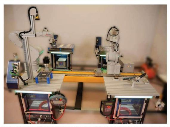
Hytech Didactic integrated Robotic Cell with Dual Robots is equipped with two 7 axes robots. This cell provides hands on experience to user on industrial integrated robotics applications. User is expected to program both robots in such a way that they work in collaboration with each other to carry out industrial processes such as deburring, polishing and engraving. Four different stations are provided to carry out various processes including storage, retrieval as well as vision inspection.
