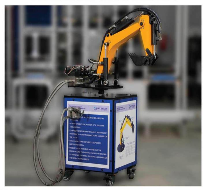
Hytech Didactic Hydraulic Excavator system is an automation module which can be integrated with any electro hydraulic training kit. Fully operational excavator system is equipped with Hydraulic solenoid valves for cylinder and hydraulic motor operation. Cylinders as well as hydraulic motor are permanently piped with the solenoid valves. Solenoid valves can be actuated with the help of 2mm Banana patch cords.
