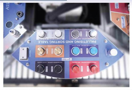
Palletising and Sorting table is provided with 16 round cells which can be utilised to pick and place round jobs which are provided along with the robocell. Each of the pocket is equipped with photosensor which gives dynamic feedback about the occupancy status of each cell.
