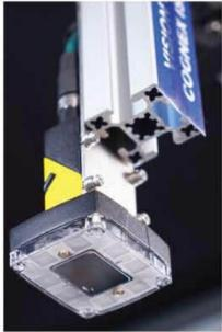
Vision Inspection table is equipped with Cognex vision sensor which can be taught to sense different shapes and provide feedback to Robot Controller / PLC.
