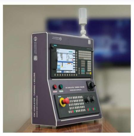
Siemens CNC Simulator is equipped with Siemens 828D Controller which comes with an option to be operated as either 2 Axes turning controller or a 3 axes milling controller. MOP as well as MPG in the Simulator is from Siemens. Tower lamp provided on the simulator can be programmed from CNC inputs and outputs.
