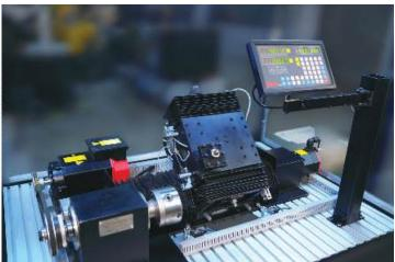
CNC Maintenance Training kits are completely different from CNC Trainer machines. CNC Trainer machines provide training on CNC Machine operations. Students as well as instructors are not supposed to change the parameters as well as the ladder of a CNC machine. CNC Maintenance Training kits are designed to provide insights of CNC Commissioning and ladder designs.
