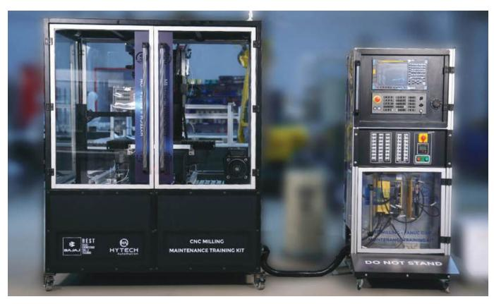
CNC Maintenance kits are designed to provide hands on experience to CNC operators or application engineers. Basic function of these kits is to experiment with the electrical panel as well as the ladder diagram of CNC machines. These training kits consist of machine slides with linear motion guideways and ball screws. Separate operation units with CNCs are provided for both turning as well as Milling maintenance training kits.
