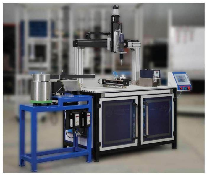
Hytech Didactic Automated **Bolt Assembly Station** can be used individually or in integration with the Computer Integrated Manufacturing Setup.
