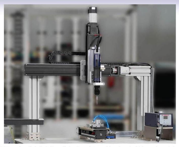
Pneumatic guided cylinder is provided on the Y axis Servo Slide to clamp the job for carrying out bolt assembly process.
