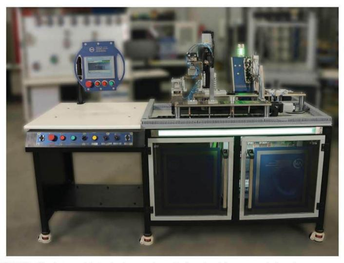
Hytech Didactic Assembly Station is a mechatronics based training system designed to carry out automated assembly of 4 different parts with pneumatically and electrically actuated process. Automated bearing dispensing station is also provided in the system. Entire station is programmed and operated with SIEMENS PLC and HMI.
