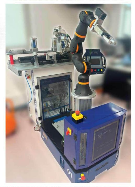
Hytech Didactic AMR Training cell is designed to provide hands on experience to students on industrial AMR applications and its integration with industrial automation components such as COBOT, PLC – HMI and Vision System.
