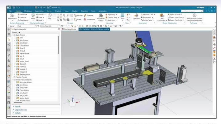
Automation station is a mechatronics based station designed to carry out colour based and weight based sorting of components. Once the sorting is completed, AMR is supposed to transport sorted job to desired position with the help of COBOT and Vision system.
