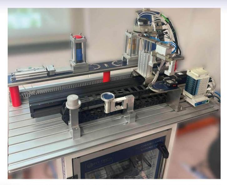
Hytech Didactic AMR Training cell is designed to provide hands on experience to students on industrial AMR applications and its integration with industrial automation components such as COBOT and PLC – HMI.
